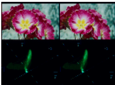
Pictures and vector scopes of Lch and Rch can be displayed simultaneously for chroma Adjustment.
